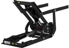
The REAC anterior tilt system is used for changing tilt angle in both directions (forwards and backwards). The system has also an additional lifting function. By applying both tilt functions at the same time, the seat is lifted vertically 202mm.
