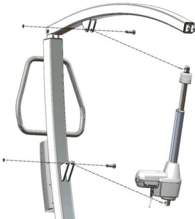
Figure 2 Mounting of RE7000
